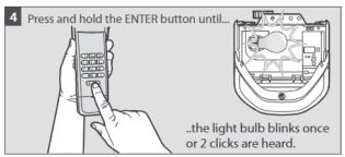
To test, press the PIN, then press the ENTER button. The garage door opener will activate. To program the Keyless Entry to more than one garage door opener, repeat the steps above using a new PIN for each additional garage door opener.
