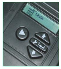
The control panel allows the installer a quick and easy way to program numerous functions simply by clicking through the intuitive menu.
