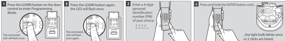
To test, press the PIN, then press the ENTER button. The garage door opener will activate. To program the Keyless Entry to more than one garage door opener, repeat the steps above using a new PIN for each additional garage door opener.
